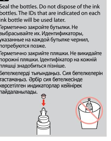
Seal the bottles. Do not dispose of the ink bottles. The IDs that are indicated on each ink bottle will be used later.
