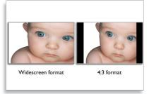
Philips easy picture format control on OSD is to switch from the 4:3 aspect ratio to the widescreen mode and back again to match the display's aspect ratio with your content for working with wide documents without scrolling or viewing widescreen media in the widescreen mode and distortion-free, native mode display of 4:3 ratio content.
