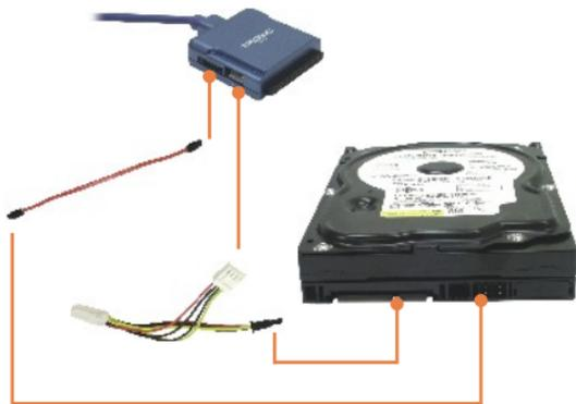
**Note:** If your SATA hard drive comes with a legacy 4-pin power connector, use the 4-pin power connector instead. To connect to both IDE hard drive and SATA hard drive with legacy 4-pin power connector, you need a 4-pin Y type power cable to convert a single 4-pin power connector into a double 4-pin power connector.
